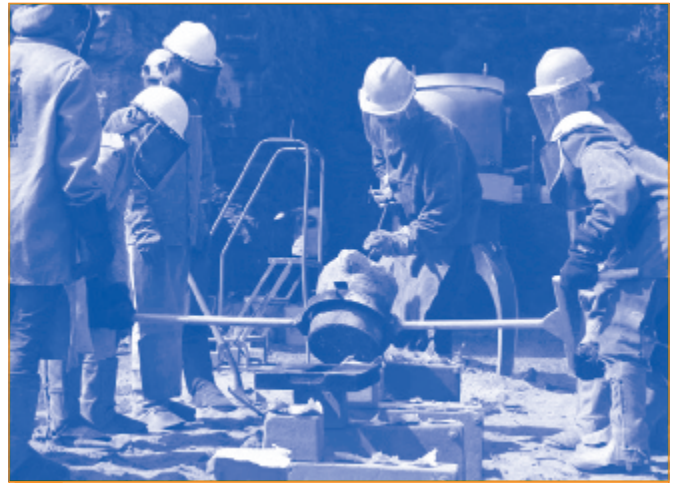
Molten iron is poured into molds as a part of the Keystone Iron Works program.
